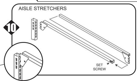
Wall stretchers are used to stabilize freestanding bays. Only the slotted end panel can be used in the application shown. However, the wall stretcher may be hooked directly into an upright with no end panel. The maximum span should not exceed 51". Once the stretcher is secured, the set screw should be tightened.
