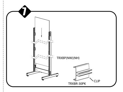
Install (2) clips at bottom of upright right above bay stretcher. Slide back panel until it rests on floor. Bow out back and attach (2) more clips approximately center of upright height. Finally install (2) more clips at top of panel right below top bay stretcher.
