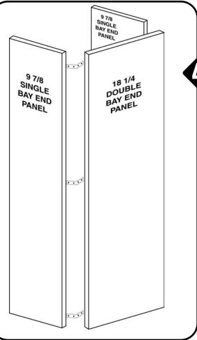
When placement for an aisle is reached, a bay end box must be constructed. Assemble the box using one double bay end panel and two single bay end panels. Use the corner hardware. **Note** that the double bay end panel is outward facing, and boxes over the edges of the single bay panels.
