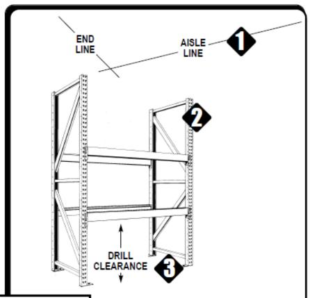
A. If using particle board deck, insert deck supports and deck on the designated beam pair to be sure section is square. See chart below for quantity of deck supports per beam length.
