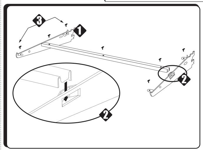
Install brackets in upright at desired height... one pair of brackets per shelf.
